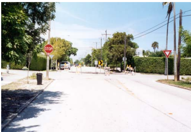
Conflicting Regulatory Signs on Opposite Sides of the Street
